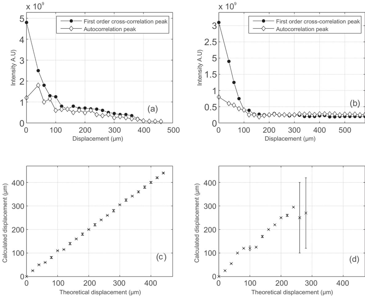
**Figure 2** (a)-(b) Criterion for reliable range of measure in horizontal and vertical sense respectively. (c)-(d) Calculated versus theoretical displacements in horizontal and vertical directions correspondingly. Data taken from reference [12]
